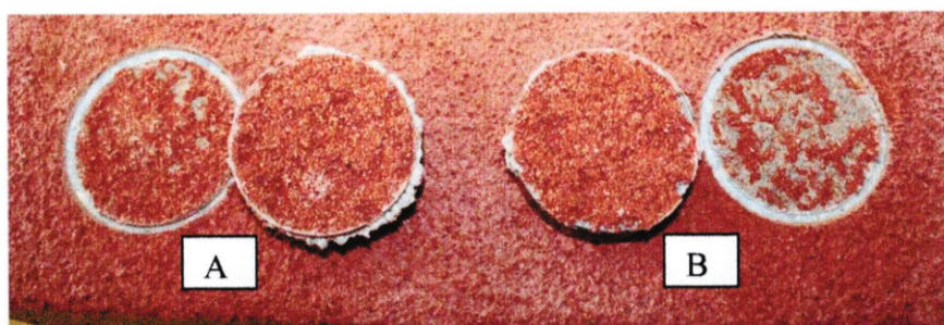
Figure 1. Surfaces separated after the adhesion test. A: 100% Cohesive failure in the sprayed cork and support B: 50% Mix failure 50% A/B – 50% B: 50% adhesive failure between the sprayed cork and the concrete support and 50% cohesive failure of the sprayed cork
